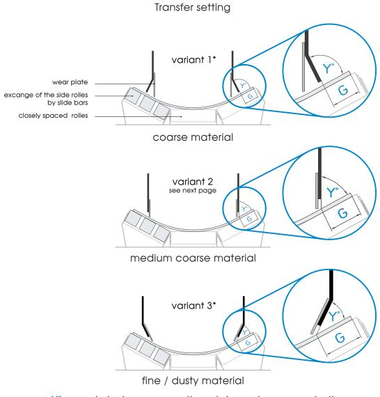
Y° = angle between mounting plate and conveyor belt \*consultation with ScrapeTec Trading GmbH
