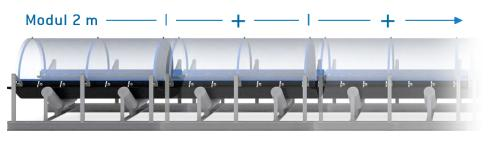
The combination of the AirScrape and a dust retaining filter cloth hood results in the DustScrape. This dust protection system is suitable for installation at free transfers or conveyor sections.
