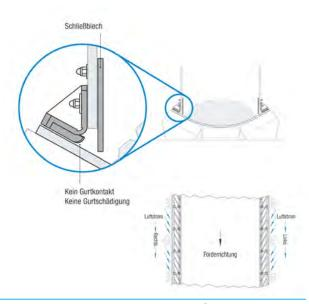
Air is sucked in between the diagonally oriented lamellas of the left and right side AirScrape elements from outside to the belt centre. It is important that the installation specifications are followed closely, in order guarantee the benefits of the system.
