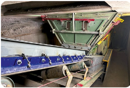
After installation: Dust and spillage reduced by 95%+ after installing AirScrape®, TailScrape & K-Containment® Seal.
