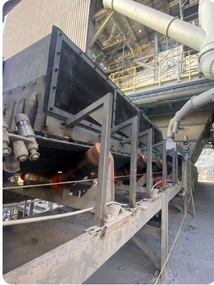
The DustScrape dust emission prevention system consists of a filter cloth, support arches and skirts, arms to hold the system above the belt and a rubber curtain to eliminate further dust development.
