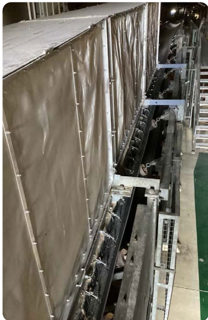
AirScrape and DustScrape combination eliminates dust and spillage plus the fire and explosion risks at the transfer chute load zone is greatly minimised.
